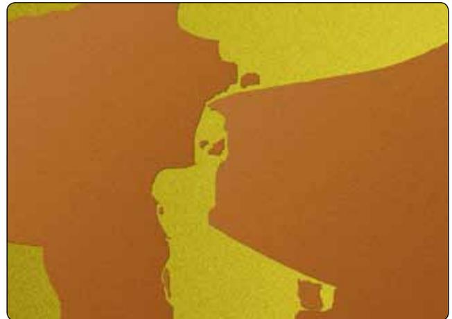
Figure 8-13. Example of poor adhesion.
